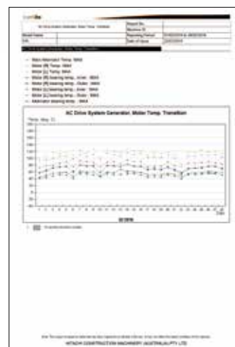
AC Drive components temperature
