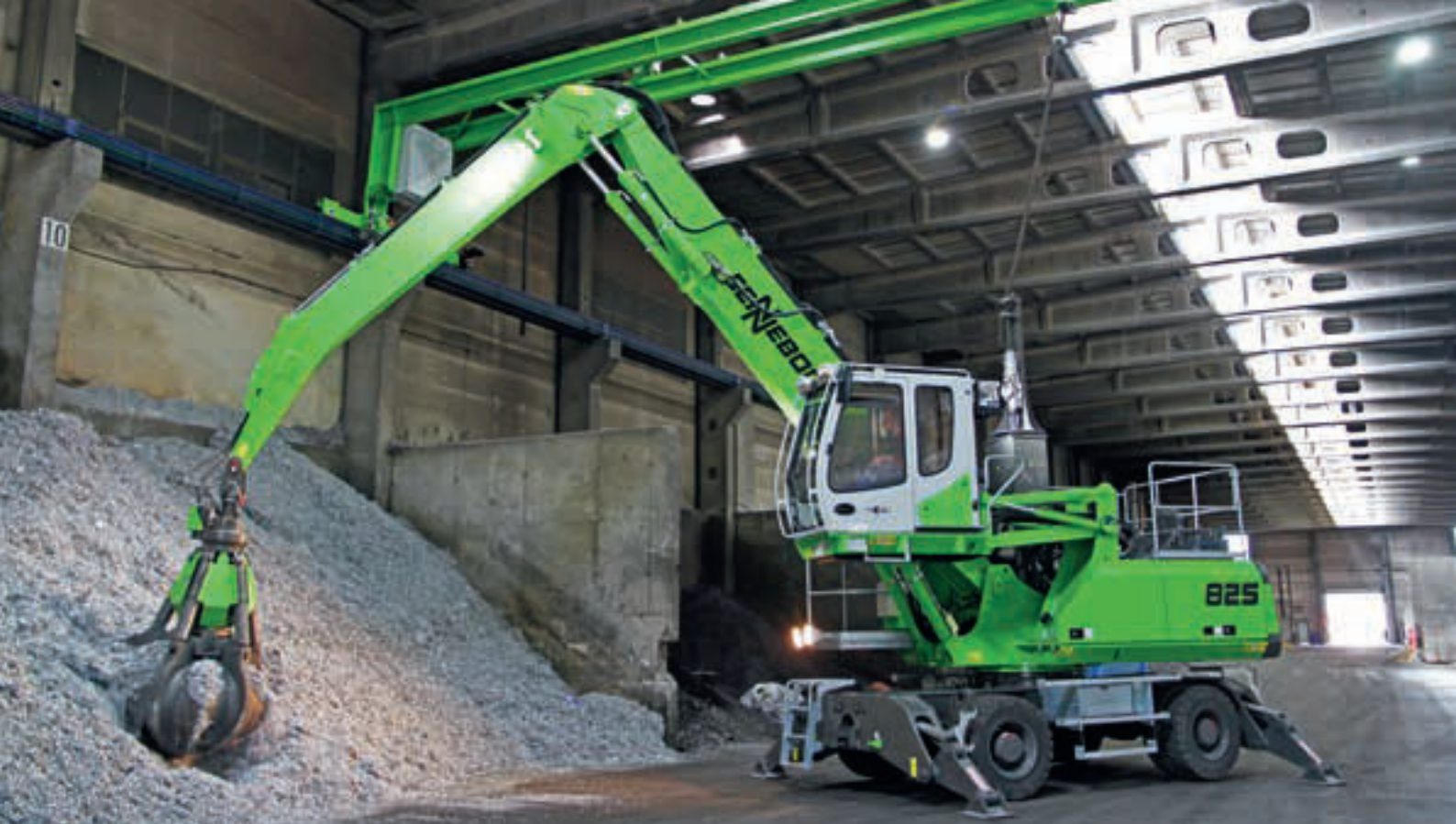
825 M Electro - Indoor scrap handling with overhead power supply; Germany
