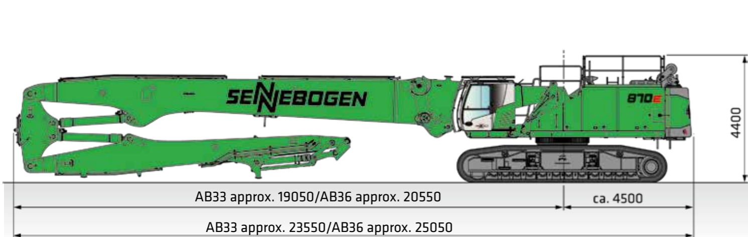
870 DEMOLITION WITH T102/420 UNDERCARRIAGE AND 3-PART DEMOLITION BOOM, HYDRAULICALLY ELEVATING MAXCAB, TILTABLE UP TO 30°, ULM OPERATING WEIGHT APPROX. 114 T - 117 T (WITHOUT TOOLS)
