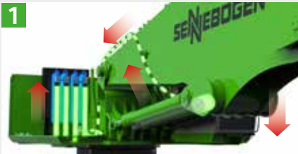
1 Boom lowers, gas compresses
