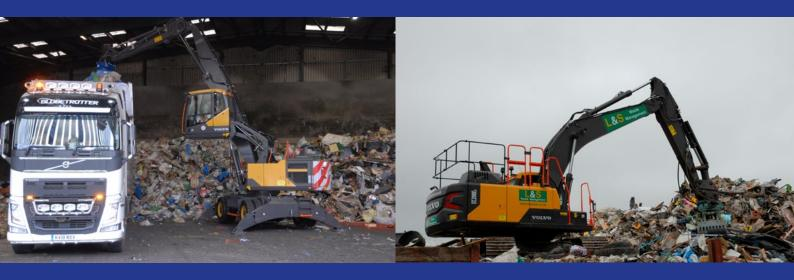
Specifically designed for waste and recycling industries, the EW240 MH is perfect for waste handling activities. This machine works a 12 hour shift seven days a week, loading either high-sided bulkers or a high capacity mobile shredder. 50,000 tonnes of waste will be handled by the machine each year. This material handler is fitted with a fire suppression system, auto-greasing system and flashing rear blue strobe lights.
