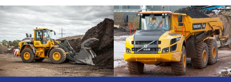
This L90H Loading Shovel is equipped with a 3m³ Hi-Tip bucket, complete with top clamp. This has been key to handling the variety, weight & density of the materials arriving on-site. This machine is also fitted with a BM AIR filtration system to filter and pressurise the air entering the operator's cab. This eliminates dust and odour arising from handling decomposing materials. The system includes an audible and visual warning if the pressure drops inside the cab.
