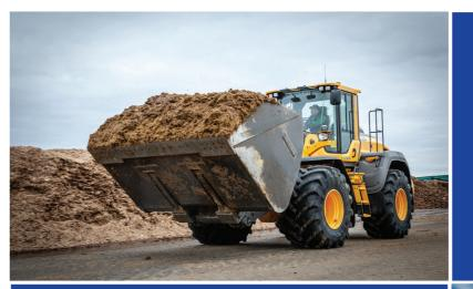
This highly specified L110H was chosen for its fuel efficiency, productivity and reliability. It features a 7m³ high-tip bucket capable of loading 100 tonnes of material into their anaerobic digester per day. The machine can easily change to a hydraulically folding grass fork for handling silage and also features 750/65 Michelin XBIB agricultural wheel and tyre assemblies which will enable the machine to work on the company's farm lands when needed.
