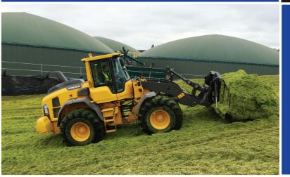
This Volvo L70H, fitted with a hydrauically folding silage fork, can ramp up and push as much as 14 tonnes a time building silage clamps. When used on grain handling duties it fills a 6m³ bucket with around 4 tonnes per load with ease. The machine is fitted with Michelin 750/65 Mega XBib wheel and tyre assemblies, additional work lights & has a reversible fan for working in the grain sheds.
