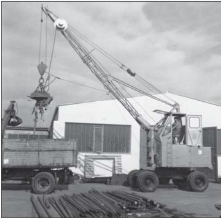
1962: rope-driven S833 with elevated operator cab
