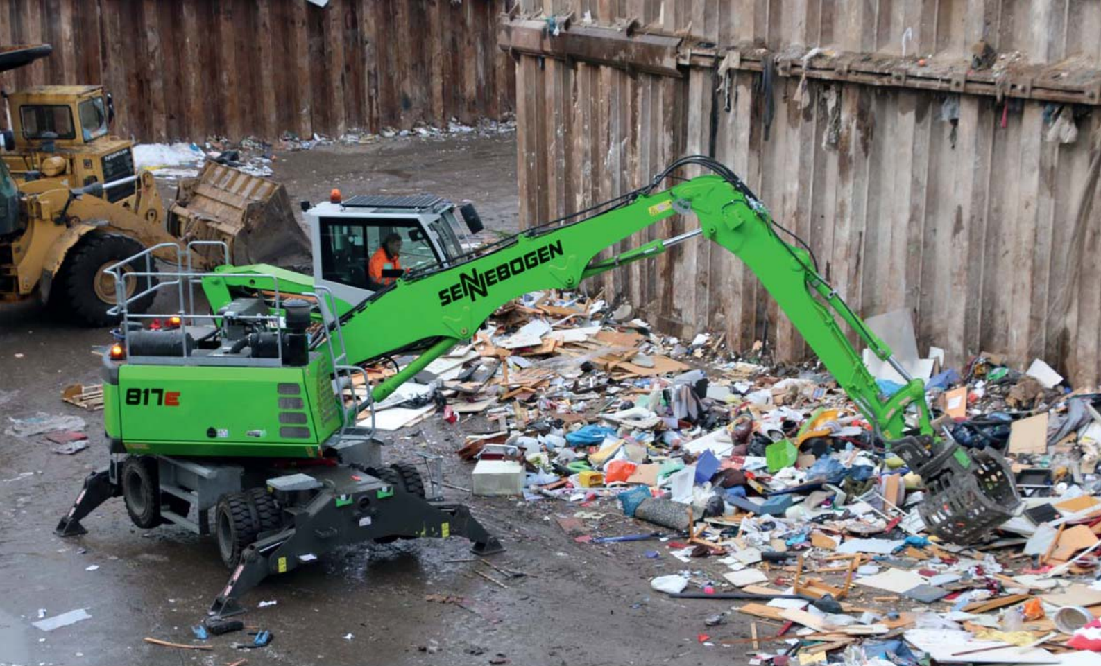
817E - modern material handler for fast and precise sorting works in waste management
