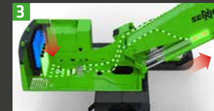
3 The nearly constant force transmission throughout the cylinder cycle supports the next boom lift
