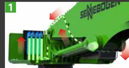
1 Boom lowers, gas compresses
